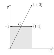
The resultant of these two is  $2\mathbf{j}$ . So, the third force must be  $-2\mathbf{j}$ . And, for rotational equilibrium, all three lines of action must pass through the same point, marked *C* above. Hence, the line of action of the third force is  $x = \frac{1}{2}$ .
