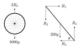
Using the dimensions of the wheel and struts, the strut is the hypotenuse of a (3, 4, 5) metre triangle. So,  $\sin \theta = \frac{4}{5}$  and  $\cos \theta = \frac{3}{5}$ .
