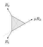
The chock is in equilibrium. Perpendicular to the slope,  $R_2 = R_1 \sin 30^\circ$ , so  $R_1 = 2R_2$ . Parallel to the slope,
